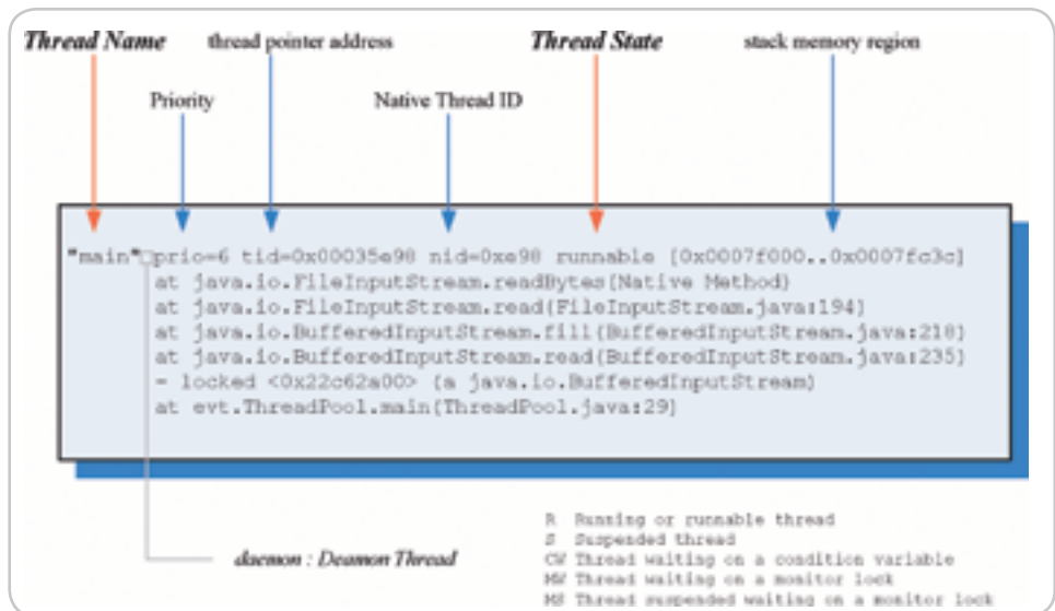
Figure 2 A sample stack trace of a thread in the thread dump
