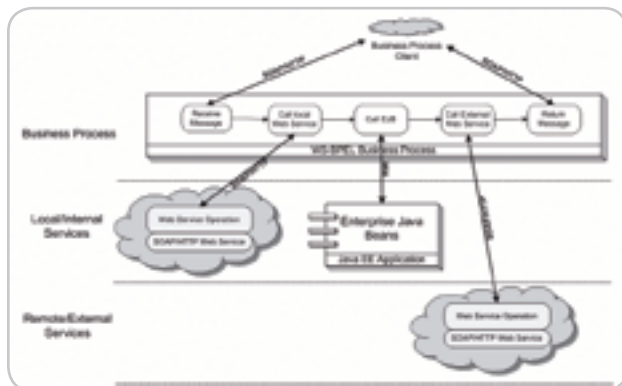
Figure 8 WS-BPEL invoking SOAP/HTTP Web services and Enterprise JavaBeans
